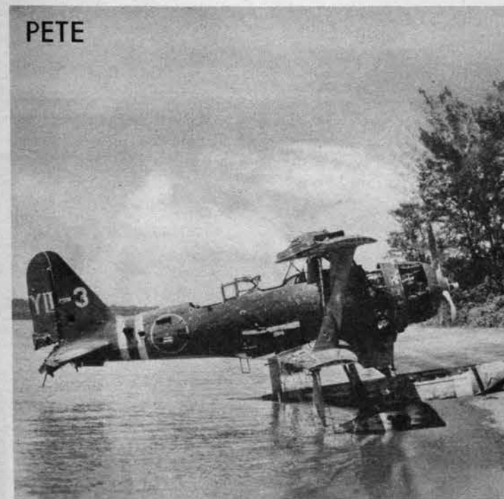
Pete is single-engine, single-float biplane used for short-range reconnaissance as is U.S. Navy's OS2U. Like OS2U, Pete operates from warships. It can carry two 220-lb. bombs and has engaged U.S. fighters.
